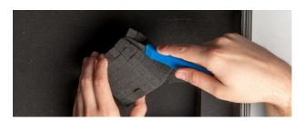
After cutting the deeper foam, remove the whole foam block, and cut it in half.
